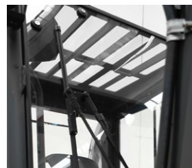
Front screen and roof with wiper / washer
